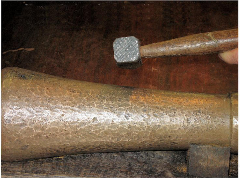
Structuring the Casting Burr Area
