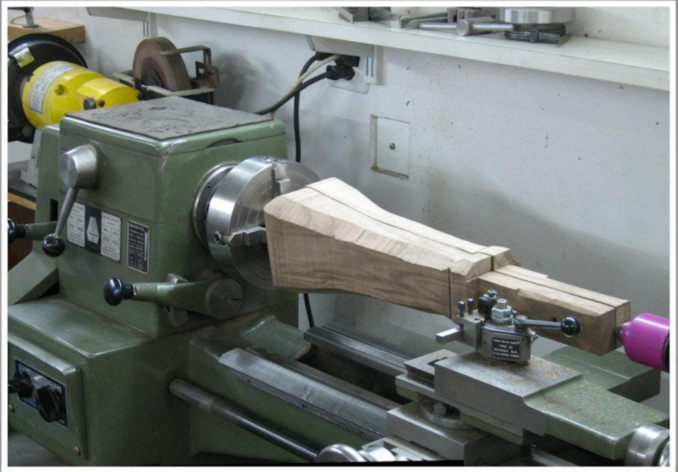
Machining of the Wooden Modell
