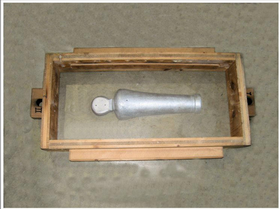
Casting Frame with Mold Half
