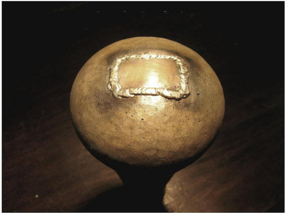
Welded Shrink Holes
