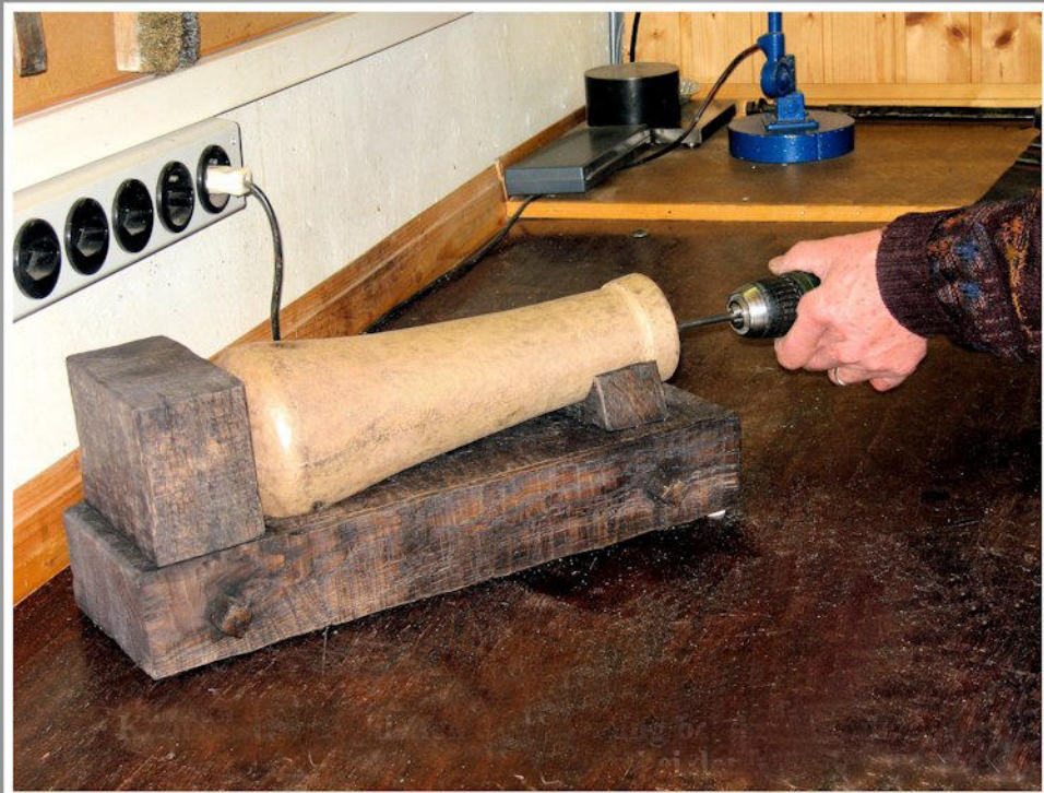
Tapping the Bore at the Muzzle
