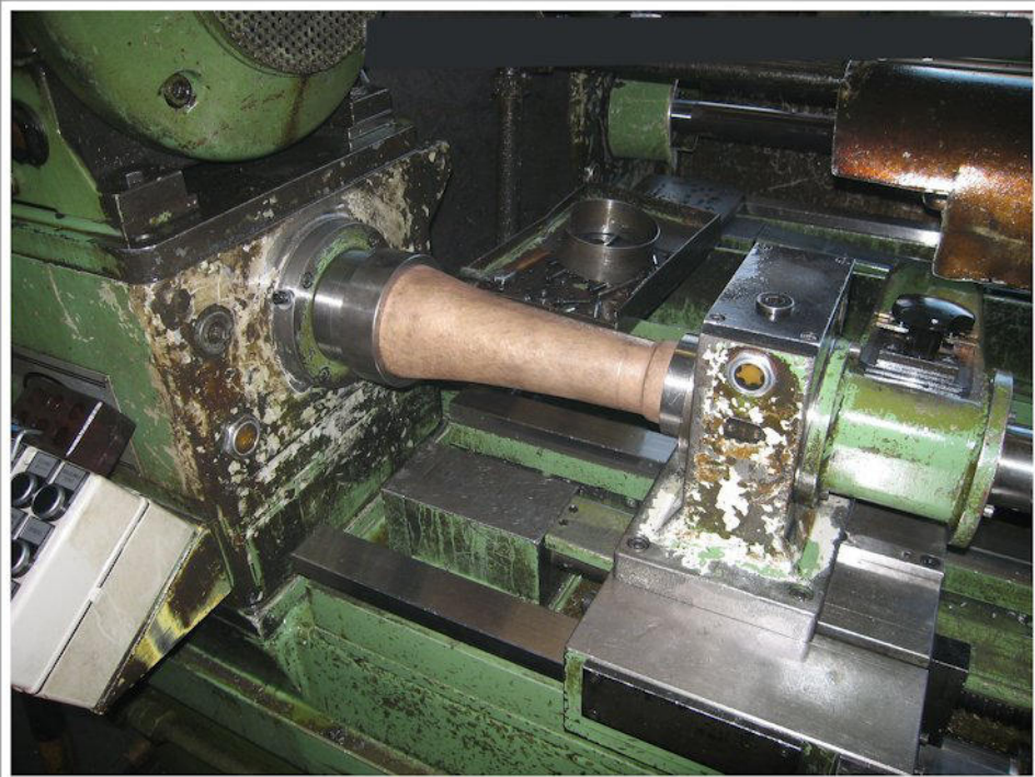
Loshult Barrel in Drilling Machine
