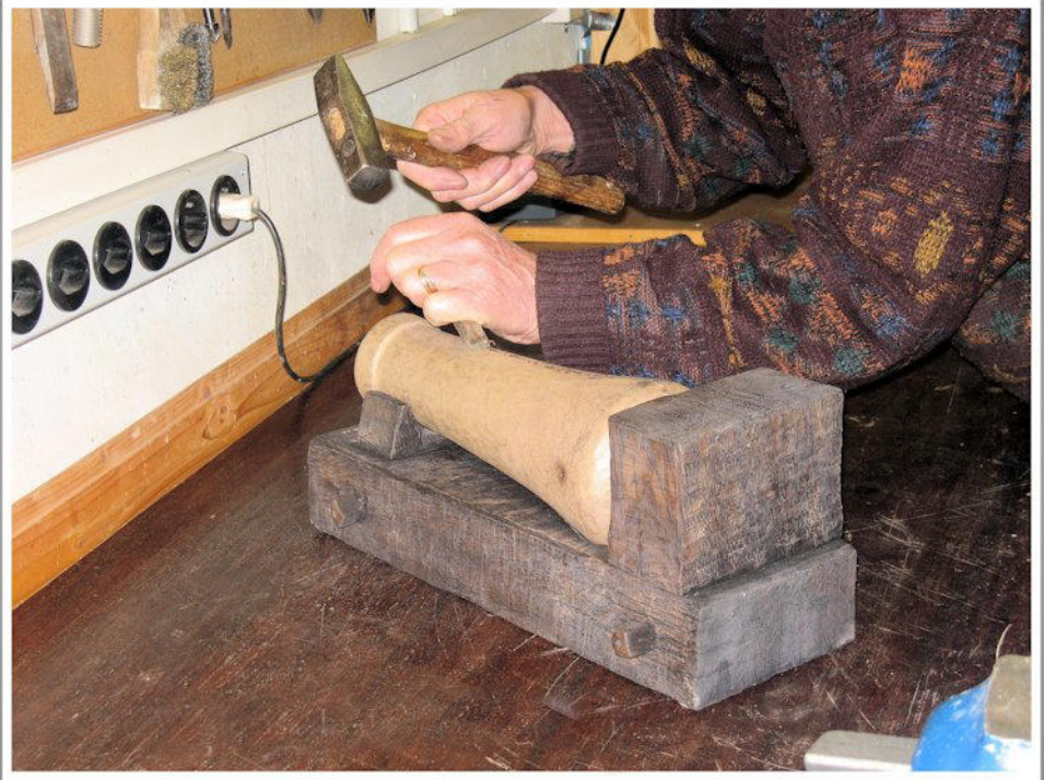
Cutting off the Casting Burr
