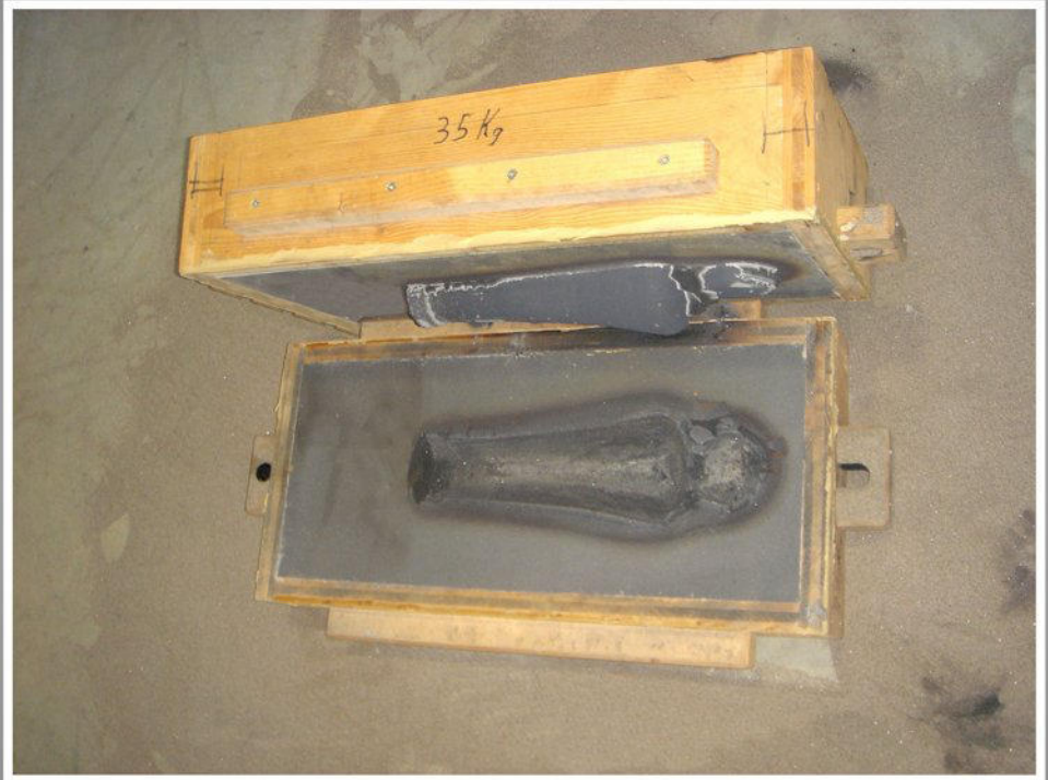
Opening of the Casting Mold
